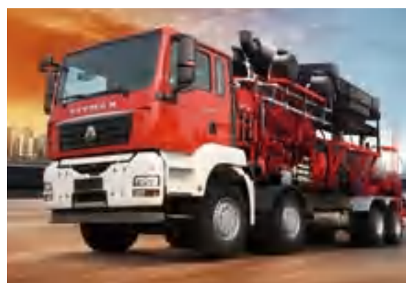
交流耐压车载试验平台底盘 CHASSIS OF AC VOLTAGE- WITHSTANDING VEHICLE TEST PLATFORM
